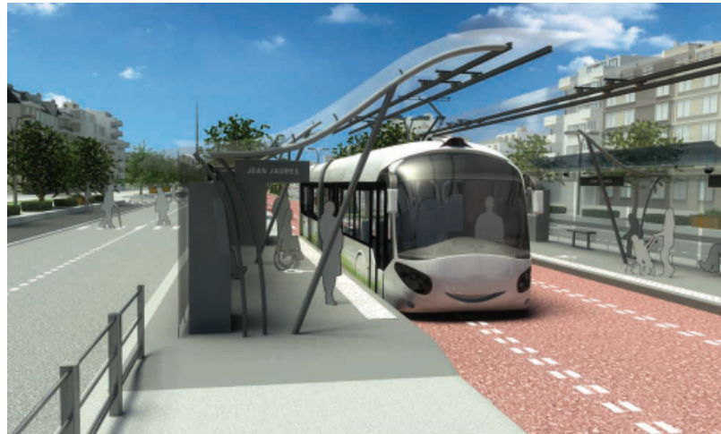
Fig. III-4.7: Charging point at a stop taking the e-BRT system from Siemens as an example
