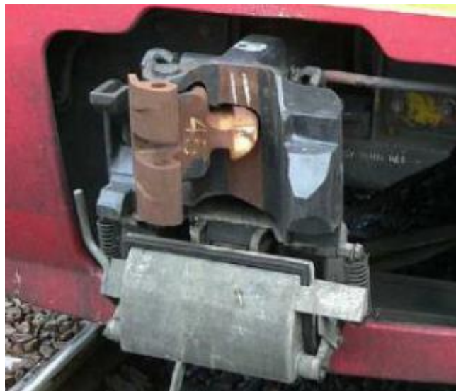
Figure 20: Automatic Tightlock coupler, provided with electric and pneumatic couplings
