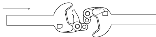
Couplers prior to connection; left knuckle is released, right one is fixed
